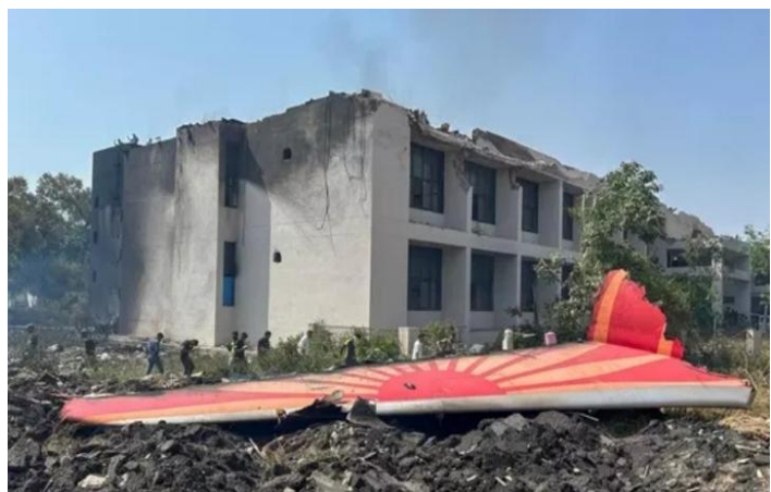
Figure 5 Vertical Stabilizer adjacent to Building A
